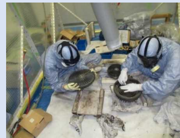
Maintenance of the scroll-pumps
