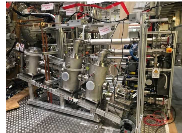
TESPEL injector German magnetic fusion experiment device, Wendelstein 7-X
