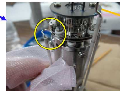
Damage of wire
