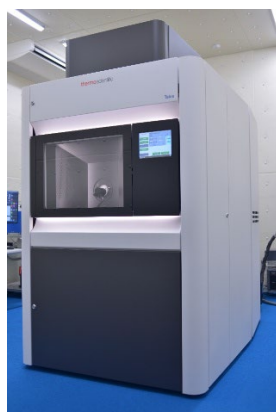
透過型電子顕微鏡 (S/TEM) (Talos F200X G2)
